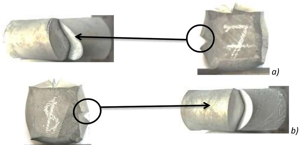
Fig. 4. General view of the braked specimens: a – specimen No. 7 ( $\epsilon = 50\%$ ,  $T_0 = 400$  °C); b – specimen No. 8 ( $\epsilon = 50\%$ ,  $T_0 = 400$  °C)
