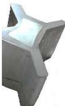
**Fig. 1. Extruded frame profile made of Al-Mg-Sc alloy (main view)**
