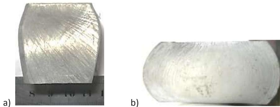
**Fig. 3. The general form of the specimen after the deformation: a – specimen No. 2 (ε = 25%, T<sub>0</sub> = 400 °C); b – No. 5 (ε = 50%, T<sub>0</sub> = 350 °C)**
