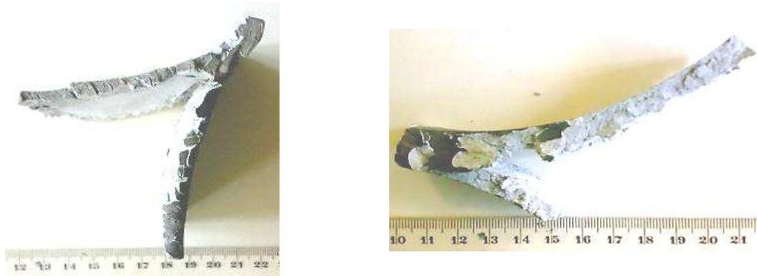
**Fig. 2. Types of breaking specimens in the rolling process**
