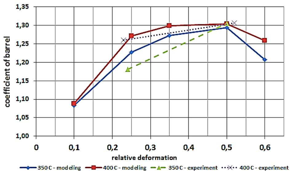
Fig. 5. Coefficient of barrel according to temperature and degree of deformation for Al-Mg-Sc alloy
